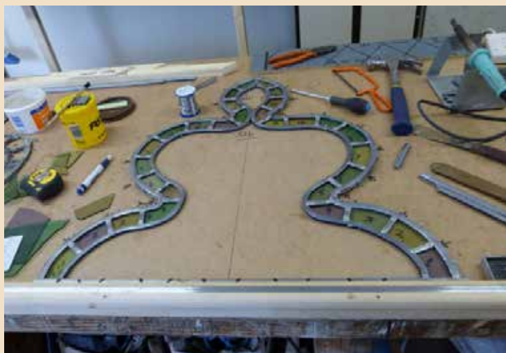
Leaded light at early stage of rebuild
